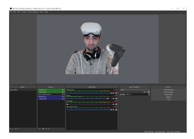
If there is a **delay between your virtual controller and your controller**, you can add a latency: right click on "Video Capture Device", select "Filters", "Render Delay". Increase or decrease the **delay parameter** according to your needs.
